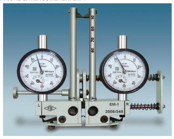
It is essential to measure the elongation of test specimen under load, to have it's mechanical properties. FIE exensometer Model EM-1 is intended to serve the above purpose.
